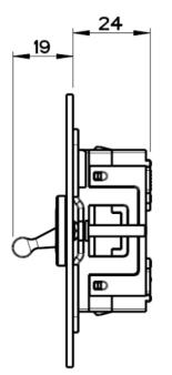
Note: plate thickness will vary between 1.5 & 2.0mm dependant on chosen finish Depths shown common to all
