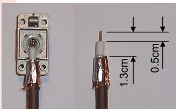
Trim back the cable as in the picture shown above. Arrange the braiding along the top and bottom of the cable to maximise contact with the screening can. Insert the centre core through the screw post and tighten, not too much that you screw straight through the wire. Shut the screening door and tighten the two screws, try not to over tighten and crush the cable excessively.
